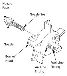
Figure 17 - Removing Nozzle
